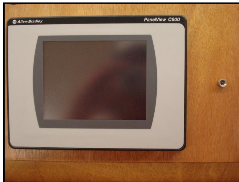
Figure 3.7. Allen-Bradley PanelView C600 monochrome human machine interface.
