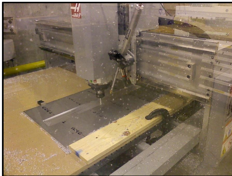
Figure 3.4. The Fryer MK 3300 vertical mill used to machine precision pieces.
