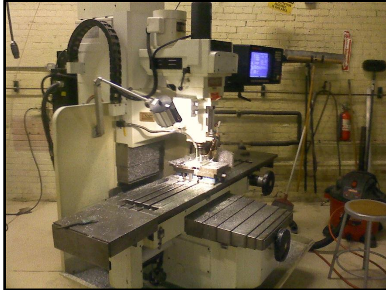
Figure 3.4. The Fryer MK 3300 vertical mill used to machine precision pieces.
